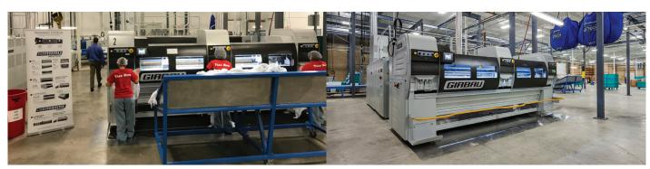
Girbau Industrial thru-station feeders automatically straighten and feed items through a corresponding ironer.
