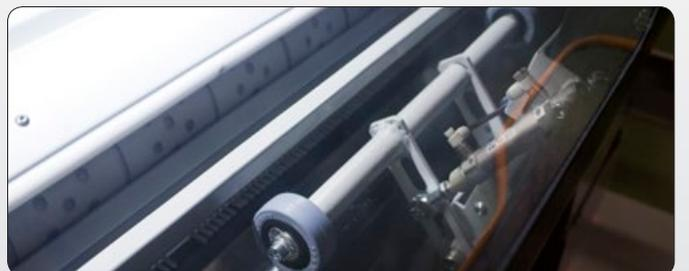
A system of compressing rollers during feeding to ensure that the item is loaded correctly, especially if it is heavy or has a tendency to slide.
