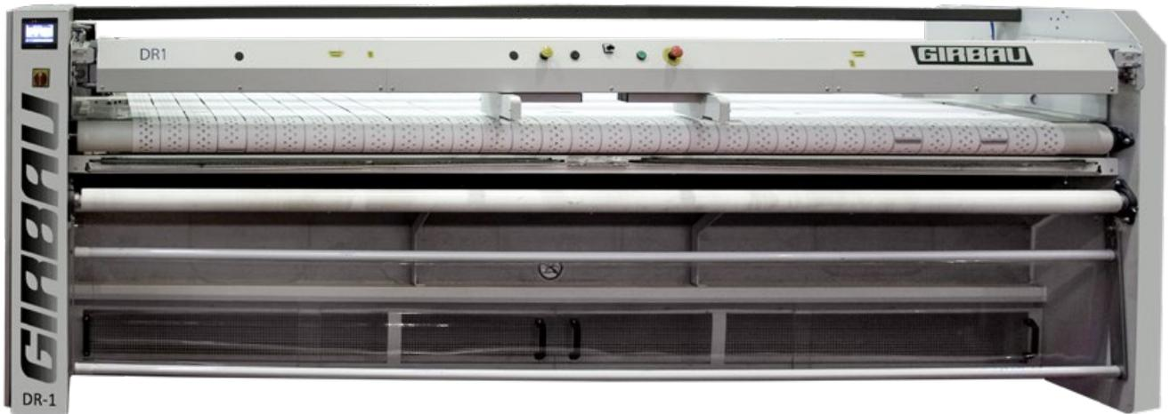
A very straightforward automatic feeder for feeding in articles automatically on 1 lane. It also allows manual feeding of items of all sizes on 1, 2 or 4 lanes.
