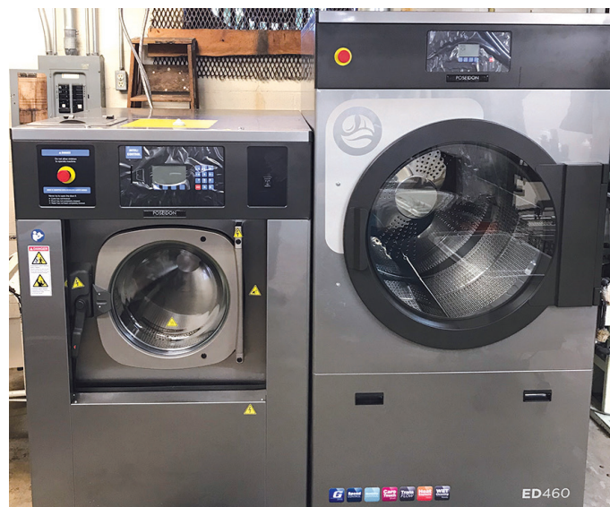
The 60-pound capacity soft-mount Poseidon Textile Care System fits easily into a space that a shirt unit and collar cuff press previously occupied. They were moved to the space previously occupied by the dry cleaning machine.
